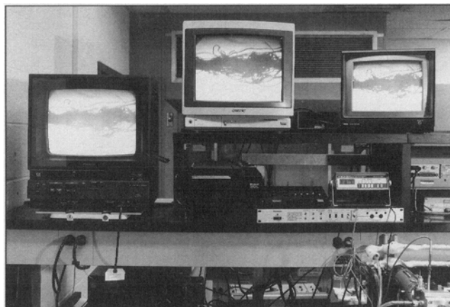
Video monitors provide close-ups for researchers to study soil removal from single strands of fibers.
