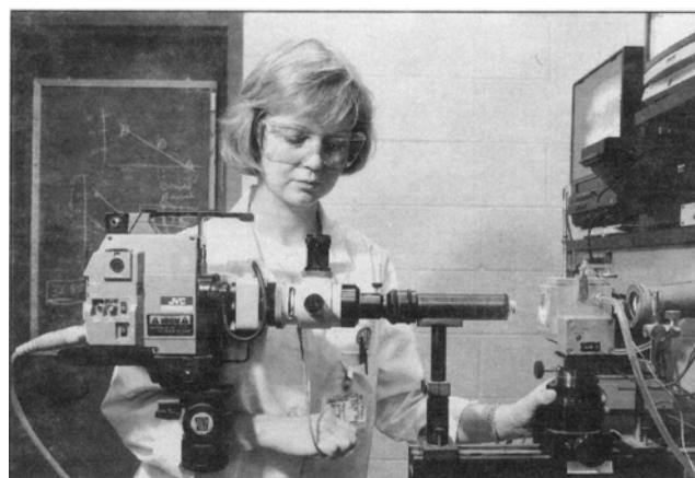
Senior research technician Leana Terrill operates a video-goniometer used in dynamic detergent studies of the removal of microdroplets of soil from single fibers.
